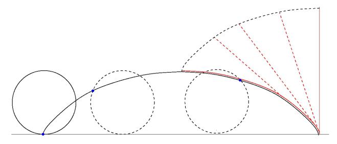
The cycloid through the origin, generated by a circle of radius r, consists of the points (x, y), with
